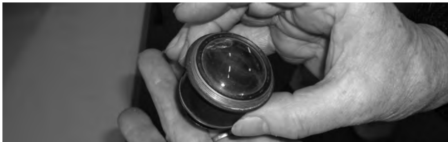
The detachable eyepiece of the Trefeca telescope.
